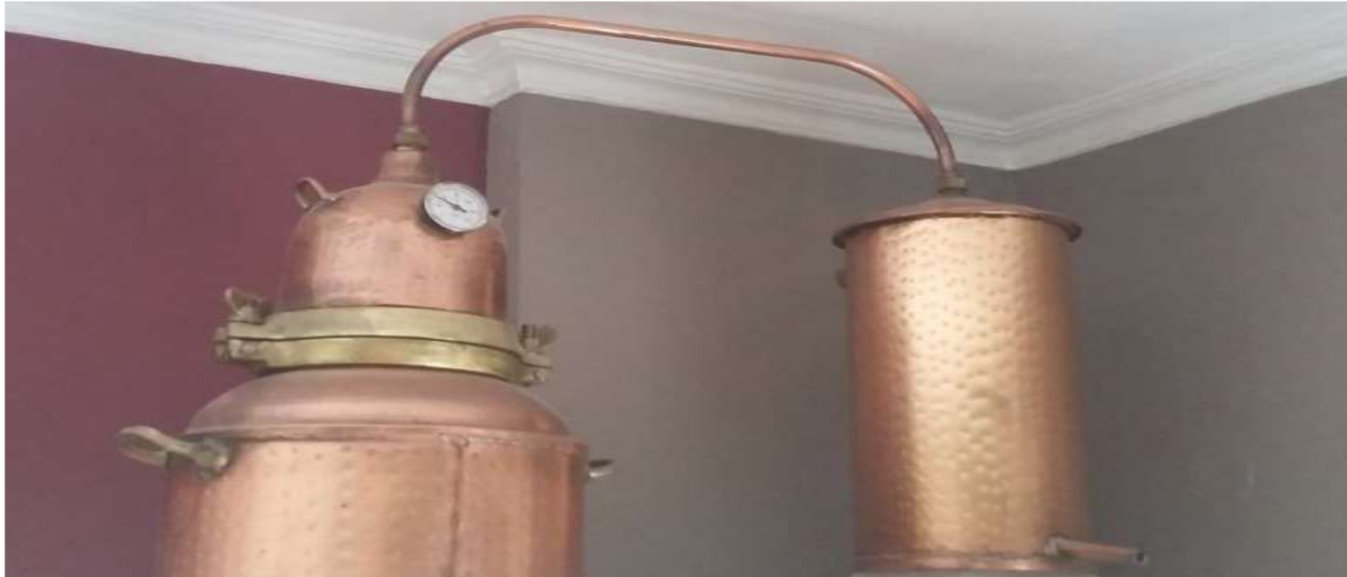
Experimental copper apparatus for the distillation of tsipouro
