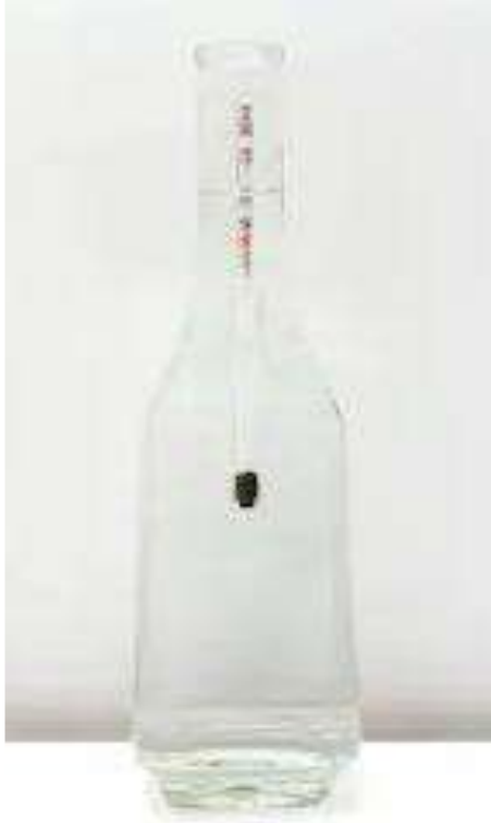
Reading the indication of the alcoholmeter on the surface of tsipouro
